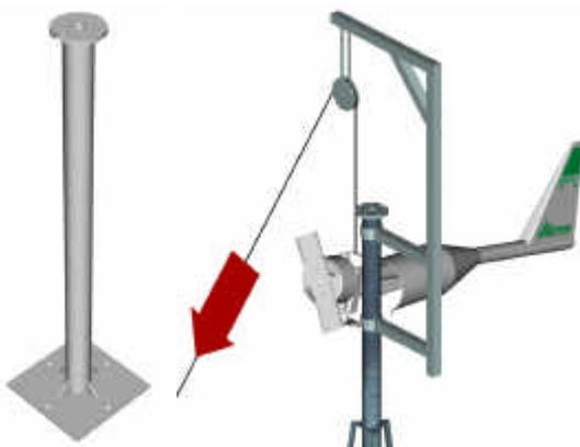
To install the wind turbine on the tower, you will need a tower adapter that will allow the blades turn avoiding crashing with the tower. Install the wind turbine once the tower adapter has been installed. It can be raised to its position using the hoist once the tower has been placed, or using a pulley system as shown on the picture.
